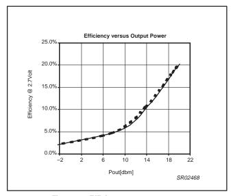
Figure 7. Efficiency vs. output power
